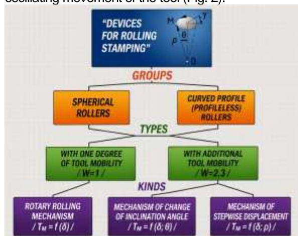
Fig. 2. Classification of devices with oscillatory movement of the tool by structural and constructive features.
