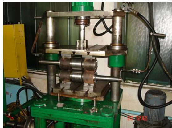
Fig. 3 - Experimental hydraulic-pulse test rig (left) and its roller technological tooling (right)
