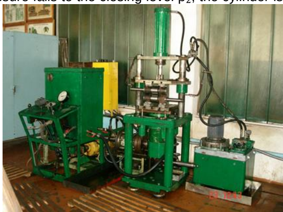
Fig. 3 - Experimental hydraulic-pulse test rig (left) and its roller technological tooling (right)
