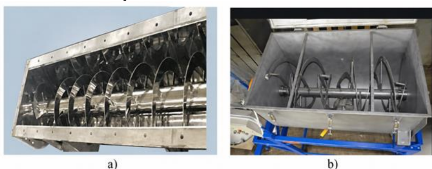
Fig. 8. Mixers with horizontally arranged ribbon screw conveyors: a) single-screw mixer; b) twin-screw mixer with oppositely rotating screws.
