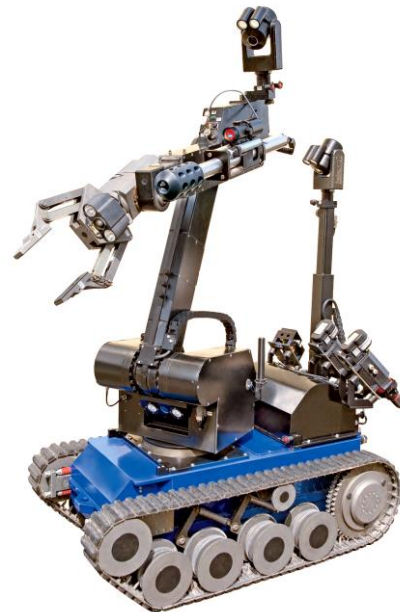
Fig. 1. General view of the terrestrial robotic complex located on a caterpillar-mover platform
