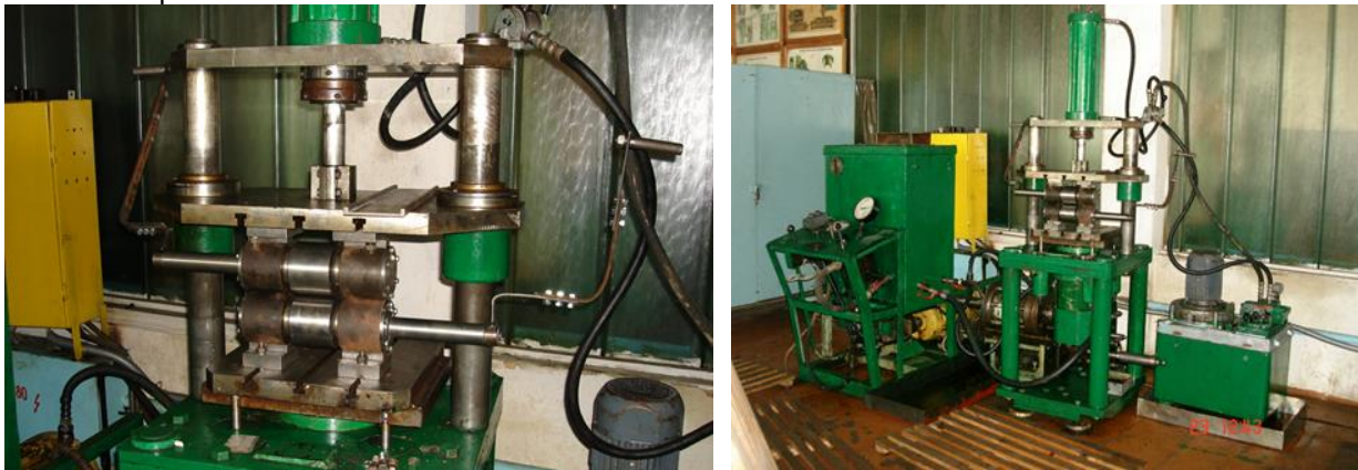
Fig. 1. Photographs of the experimental hydroimpulse stand for vibratory impact dewatering of wet dispersed materials and its technological tooling
