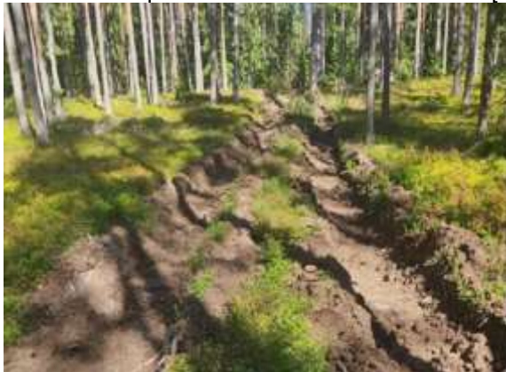
Fig. 5. A deep track left by a wheeled forest machine in one pass
