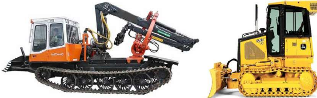
Fig 4. Visual comparison of the chassis of forestry and construction tractors
