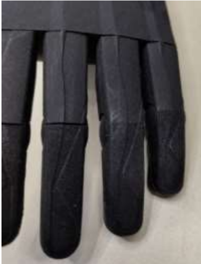
Fig. 1. Allbionics TR bionic prosthetic hand showing visible signs of surface wear after use
