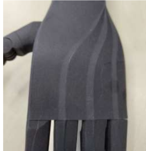
Fig. 1. Allbionics TR bionic prosthetic hand showing visible signs of surface wear after use
